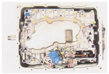
Remove the 12 valve body bolts.
