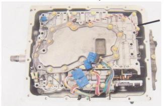
Reconnect wiring loom.
