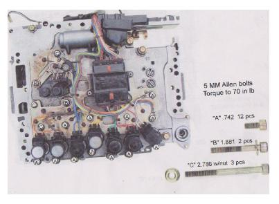
Fit Solenoids, Inhibitor switch and module And make sure the valve body is the same as the new valve body
