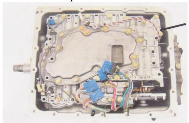
Unplug the wiring connector/s.
