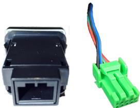
The green connector from the Module Loom must be connected to the OEM Style Switch. Ensure that the grooves on the top of the green connector align with the grooves in the hole on the back of the OEM Style Switch.
